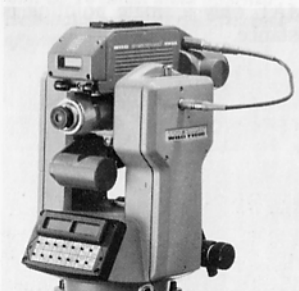
Fig. 7 Cable linking Theodolite and DISTOMAT DI4/DI4L
