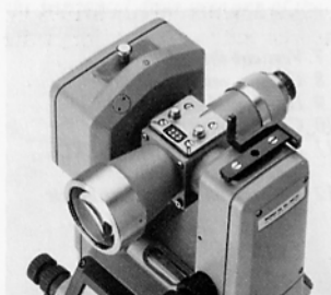
Fig. 5 Relief pin for DI3000, DIOR3002
