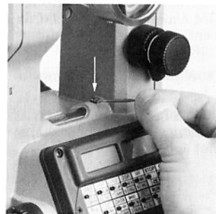
Fig. 18 Adjustment of plate level
