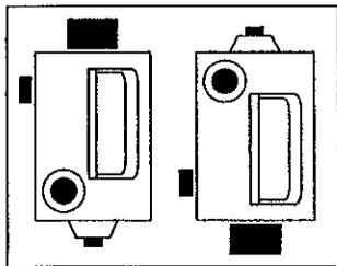
Fig. 13-2 Bull's-eye bubble is out of adjustment
