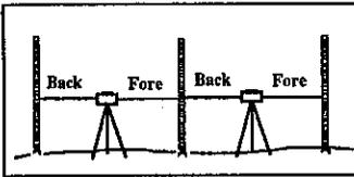
Fig. 6-2 Line levelling
