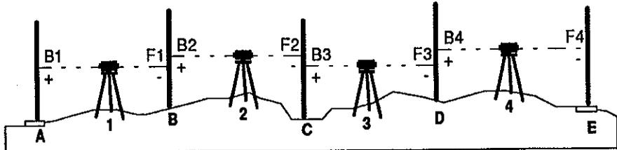
Figure 4 Line levelling between A and E
