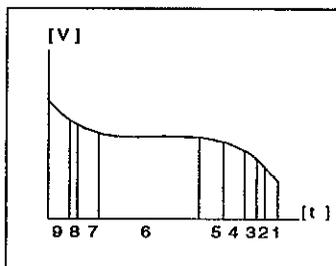
Fig. 14-3 Discharge curve for a NiCd battery
